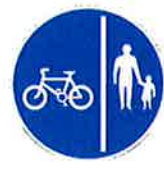
Diag No 957 Route comprising two ways, separated by the marking shown in Diag No. 1049 or 1049.1 or by physical means, for use by pedal cycles only and by pedestrians
