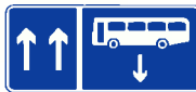
Diag No 960 Contra-flow bus lane. Note: Any vehicle may enter the bus lane to stop, load or unload where this is not prohibited. (Cycle symbol may be added below the bus symbol)
