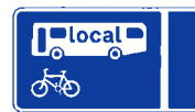
Diag No 956 With-flow bus lane which pedal cycles may also use. Note: Any vehicle may enter the bus lane to stop, load or unload where this is not prohibited
