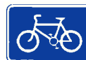
Diag No 952.1 Cycle lane on road at junction ahead or cycle track crossing road
