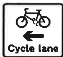
Diag No 962.1 Cycle lane on road at junction ahead or cycle track crossing road
